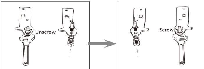
8. Refit the bracket fitting the bottom hinge pin. Replace both adjustable feet. Transfer the lower door to the property position.
