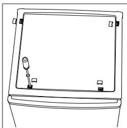
2. Unscrew top hinge and then remove upper door and place it on a soft pad to avoid scratch.
