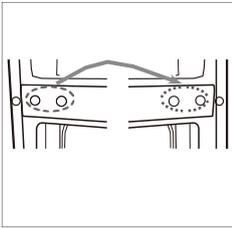
6. Unscrew bottom hinge. Then remove the adjustable feet from both side.
